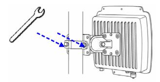
3. Adjust the antenna for appropriate tilt / vertical orientation.
